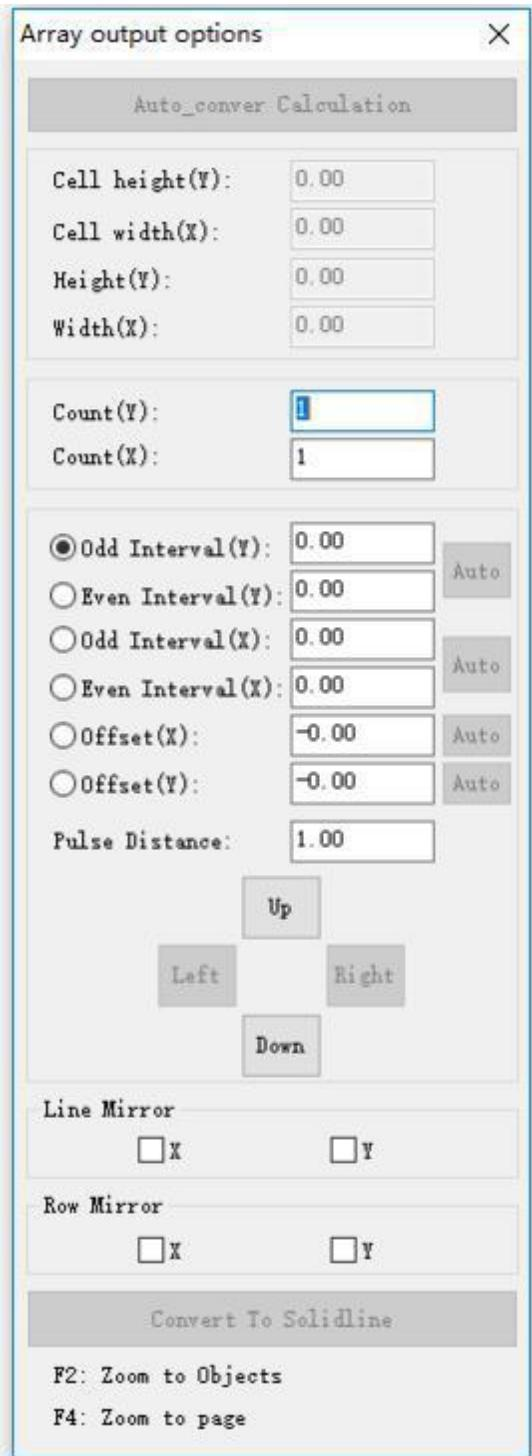
Click 【Auto cover Calculation】 , the LaserCAD software can cover the whole platform automatically with the selected graphics according to the work range and graphics size, by the most economical consumable way.
