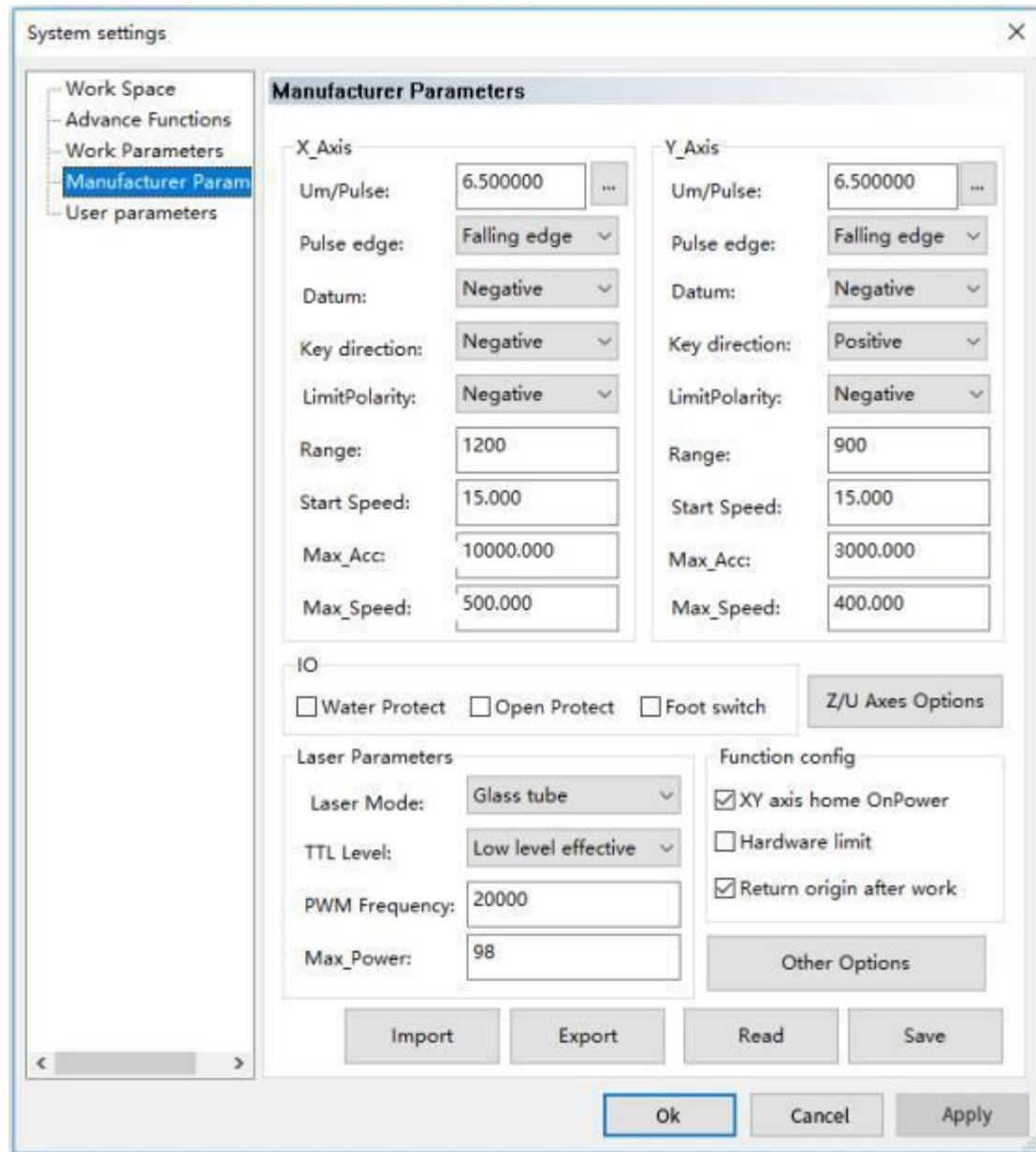
Z axis is lifting axis, U axis is feeding axis. Click **【Z/U Axes Options】** to set the parameters of Z axis and U axis.
