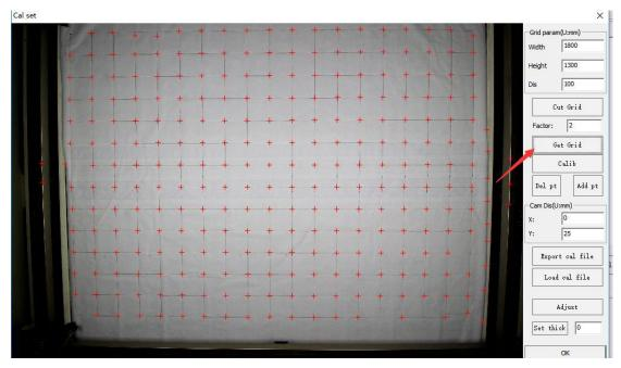
As shown in the above figure, there are extra cross points and points that are not at the intersection of the cut lines. Click on the delete point frame to select the extra cross points to delete. In the figure, the intersection of the cut lines has no cross points. Click on the acquisition point to move the mouse to the intersection of the cut lines. Double click the mouse.
