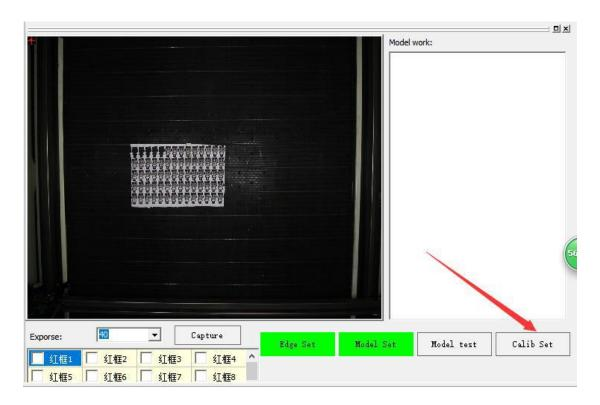
After entering the calibration management, click to get the grid point. At this time, the camera will take the photo as shown below (Remarks; click to get the grid point to take the photo. There is no calibration file in the software or the calibration file can not be used. If there is a calibration file, just refocusing is directly
