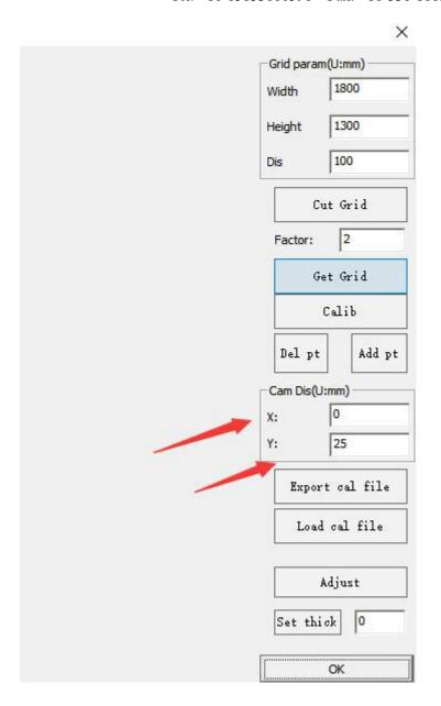
The overall deviation of the graph is adjusted to correct the distance. (Remarks; when adjusting the value, we first add the value of X Y and then cut the graph. If the error value becomes larger, we subtract the value of X Y until the cutting line graph is consistent)
