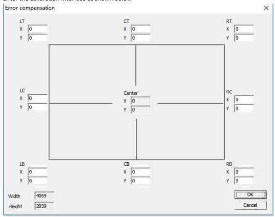
When there is a deviation in that position and adjust the value of XY of that position (Remarks; XY value adjustment first unified first and then cut the graph to see if the deviation is increased or decreased, if the increase indicates that the adjustment is reversed then adjust again)We get as shown below
