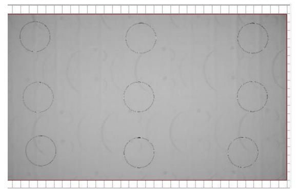
The cutting lines and graphics in the figure are offset and not completely reattached to the graphics. At this point, we click on the calibration management to enter the calibration management interface to adjust the value of X Y in the distance.
