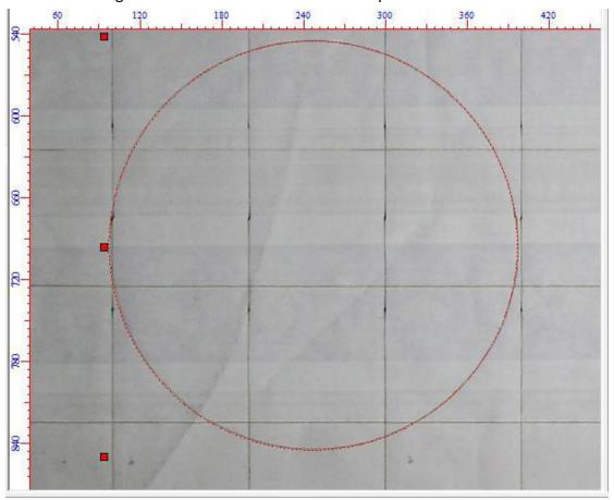
When the cutting line cannot overlap with the figure, please re-calibrate according to the above steps. When the cutting line can coincide with the figure, the paper can be removed after the calibration is successful.
