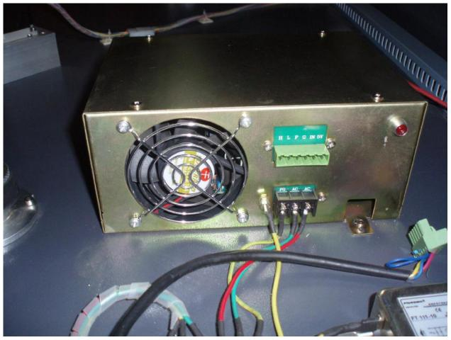
Turn off the laser machine, unplug the green 6-wire terminal on the power supply, and then turn it on.
