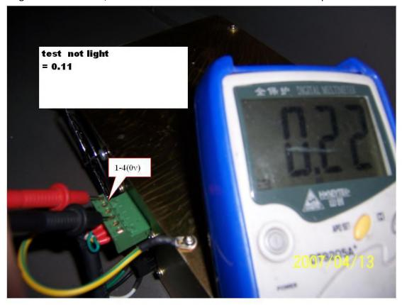
2-4: Controlling the transmition of the laser manually, you can press the "TEST" button on the operation panel.
